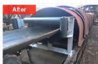
The function of the holding roller and guide roller suppresses mistracking caused by the floating of the belt, thus realizing stable running.
