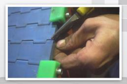
After inserting the rods, use pliers to lock the locking nail
