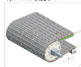
Type 型号: HS-700B Pitch 节距: 27.2MM Thickness 厚度: 8.7MM Open area 开孔率: 38%
