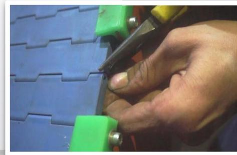
After selection of the conveyor belt which needs to be removed, disassemble it based on the above instruction, and then assemble it
