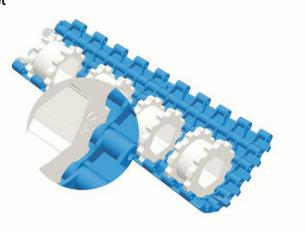
Pleaseinstall the sprocket according to the graphical representation.
